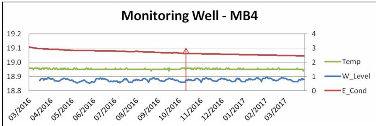
Figure 4.6: Correlation between water level, groundwater temperature and electrical conductivity in Monitoring Well MB4 during the whole monitoring period. The start of MAR is indicated by the red arrow in the plot.
