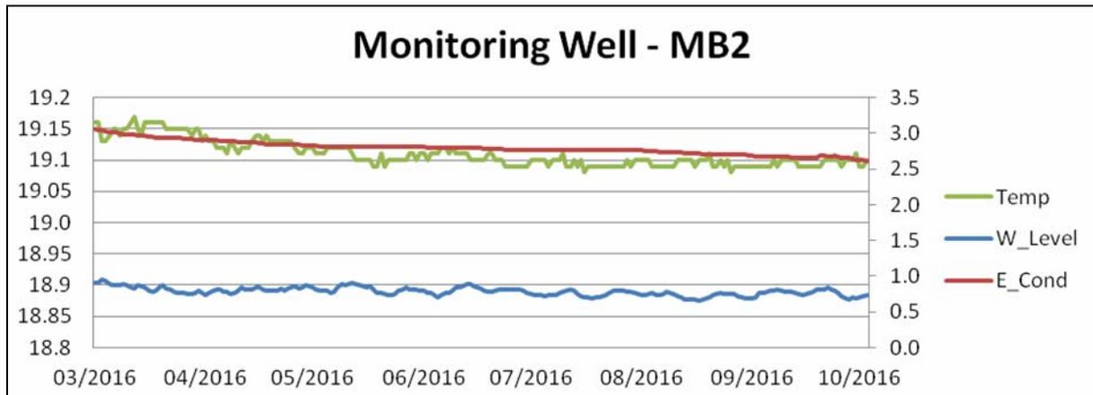
Figure 3.6: Correlation between water level, groundwater temperature and electrical conductivity in Monitoring Well MB2.
