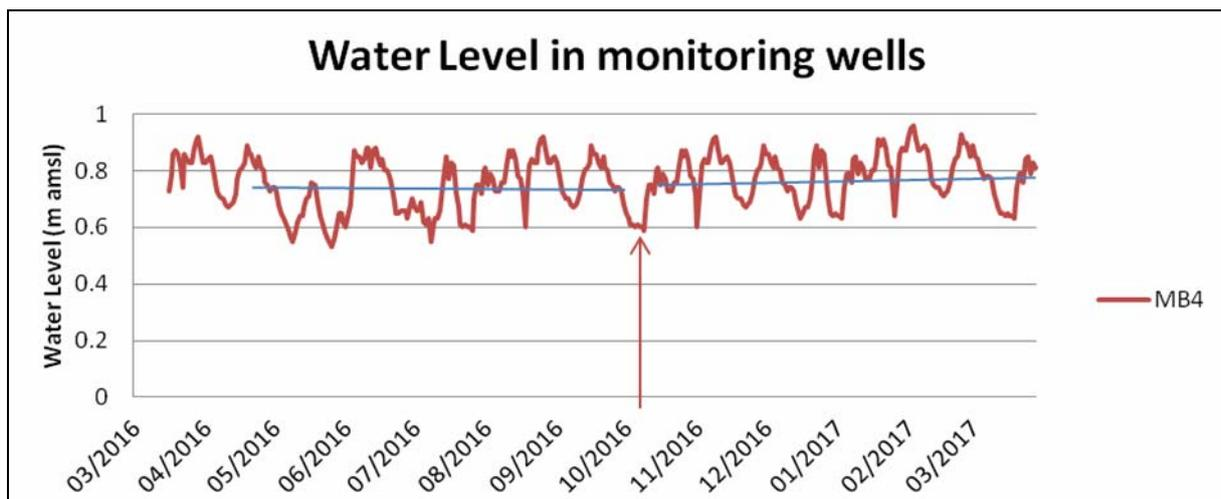
Figure 4.2: Water level readings at Monitoring Borehole MB4 which indicates an increasing tendency in water levels following the start of the MAR exercise.
