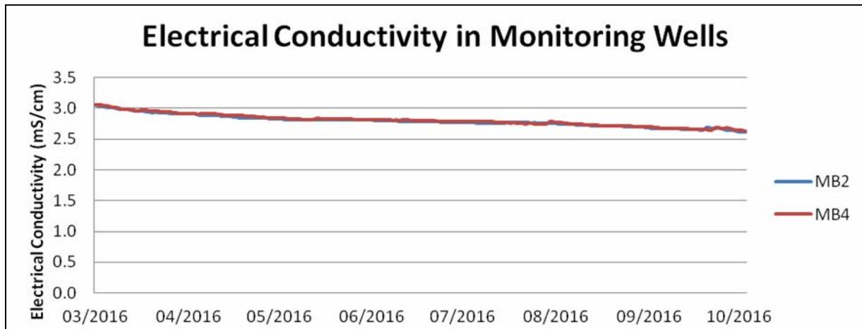
Figure 3.4 Variation in Electrical Conductivity level (at a fixed depth) in monitoring wells.
