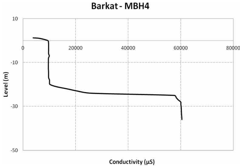
Figure 3.3: Electrical Conductivity profile along monitoring well MB4.
