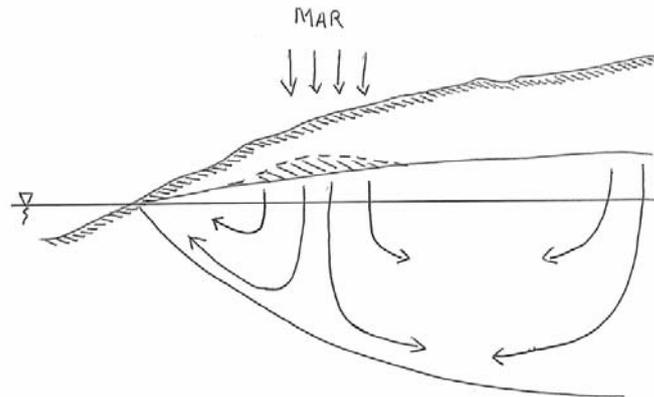
Figure 2.3: Impact of a MAR scheme in a coastal aquifer system as a sea-water intrusion barrier and improvement of quality in the downstream region of the aquifer system.
