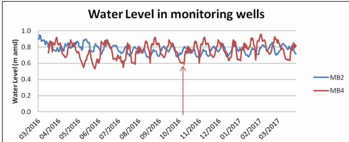
Figure 4.1: Water level readings at Monitoring Boreholes MB2 and MB4 between March 2016 and 2017. The start of MAR is indicated by the red arrow in the plot.
