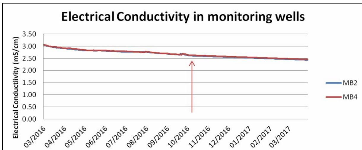
Figure 4.3: Variation in electrical conductivity level (at a fixed depth) in monitoring wells following the start of the MAR exercise. The start of MAR is indicated by the red arrow in the plot.
