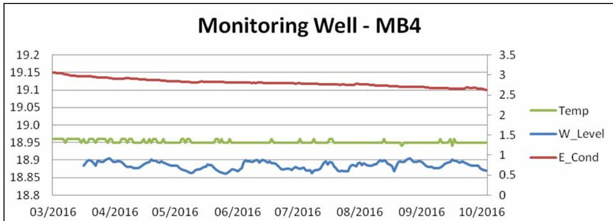
Figure 3.6: Correlation between water level, groundwater temperature and electrical conductivity in Monitoring Well MB4.
