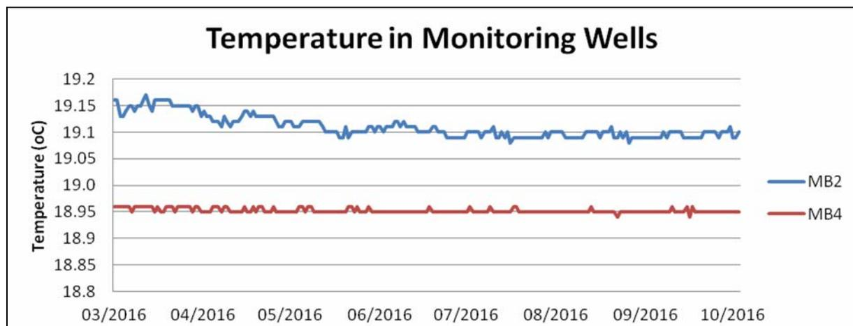
Figure 3.5: Variation in Temperature (at a fixed depth of 15m below MSL) in monitoring wells.
