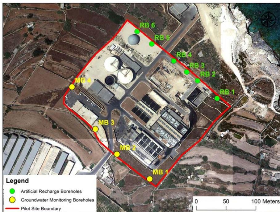
Figure 3.1: Layout of the MAR Site at the Ta Barkat Plant, indicating both recharge wells (RB1-6) and monitoring wells (MB1-4).
