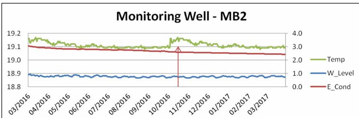
Figure 4.5: Correlation between water level, groundwater temperature and electrical conductivity in Monitoring Well MB2 during the whole monitoring period. The start of MAR is indicated by the red arrow in the plot.
