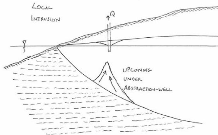
Figure 2.2: Localized Intrusion of Sea-Water beneath an abstraction well in a coastal aquifer system.
