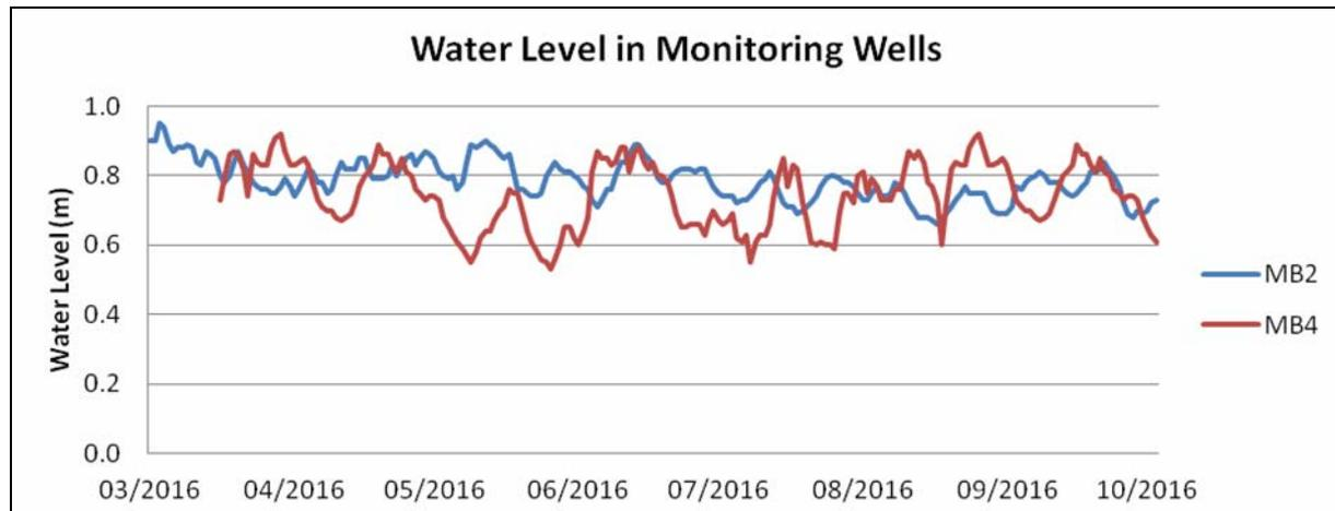
Figure 3.2: Water level readings at Monitoring Boreholes MB2 and MB4 between March and October 2016.
