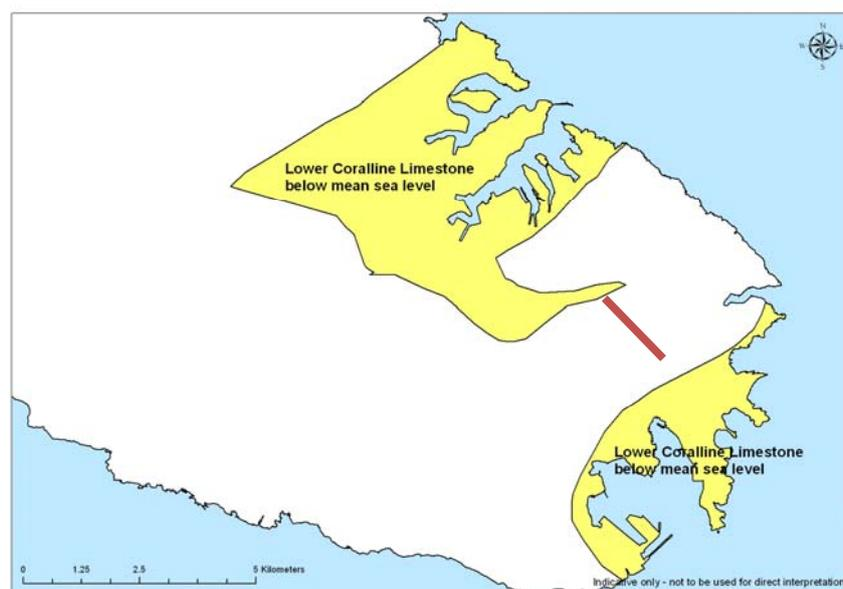
Figure 5.1: Planned up-scaled MAR site in the Malta South mean sea-level aquifer system. The red line indicates the location of the proposed MAR site.
