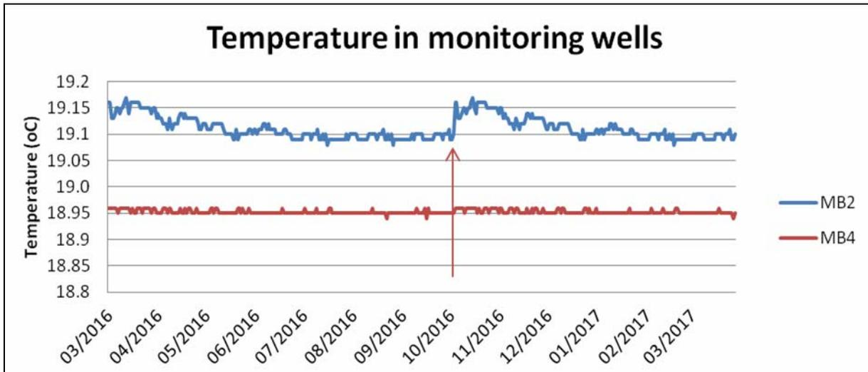
Figure 4.4: Variation in Temperature levels (at a fixed depth of 15 m below MSL) in monitoring wells following the start of the MAR exercise. The start of MAR is indicated by the red arrow in the plot.
